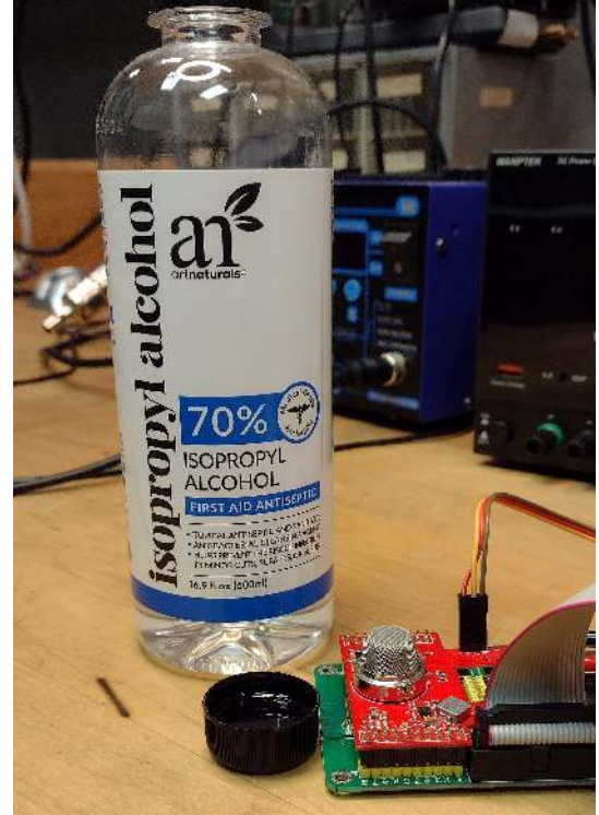
Figure 25: Using Isopropyl Alcohol as sensing phenomena for MQ135. Alcohol bottle cap filled with alcohol and placed next to sensor (b).
