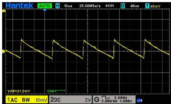
Figure 47: Voltage Ripple of 3.3 V Switching Regulator(Left) and 3 V LDO output (Right).
