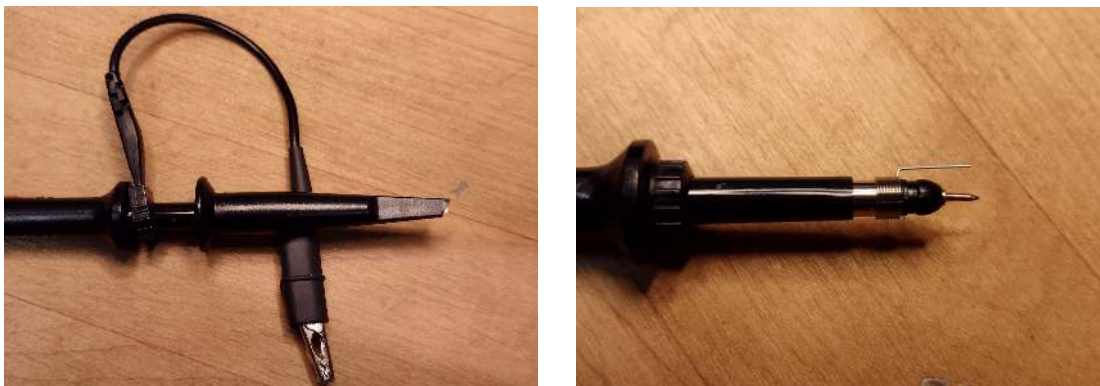
Figure 41: Replacing the Ground Lead on Oscilloscope with Ground Spring.
