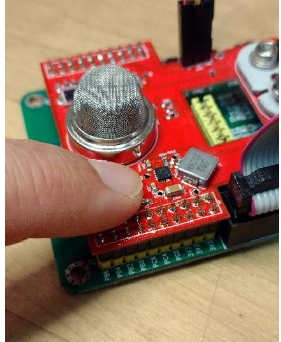
Figure 26: Touching the BMP280 Sensor to increase measured temperature.
