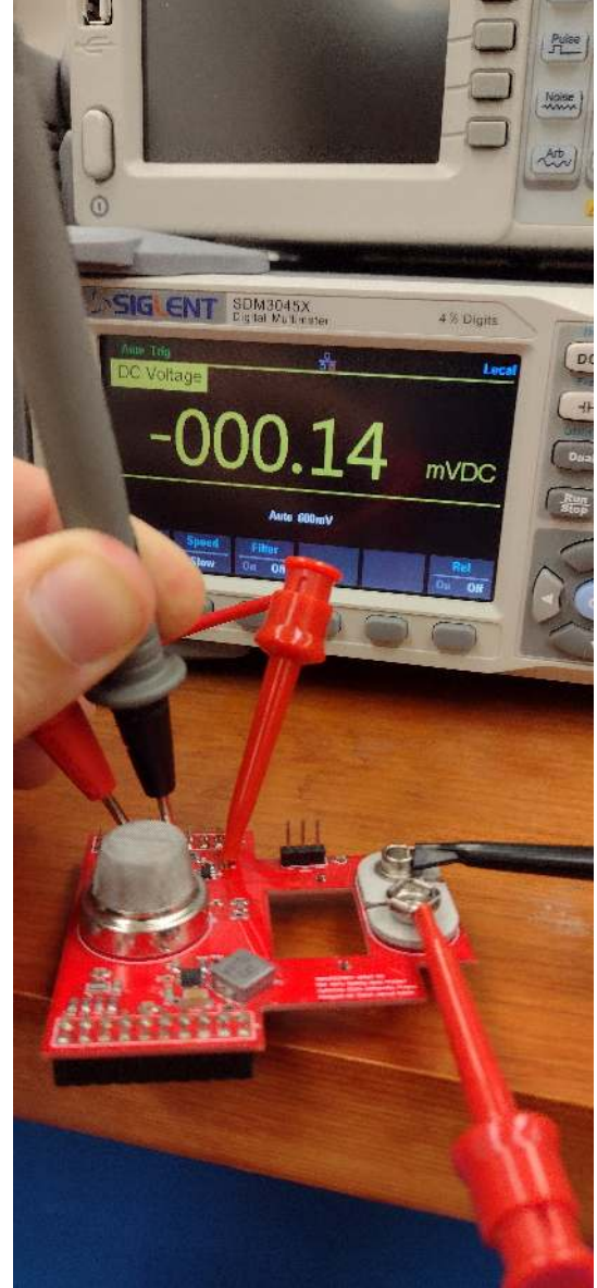
Figure 22: Voltage Reading of the 5 V Step-Down Converter with enable pin high (a) and enable pin low (b).
