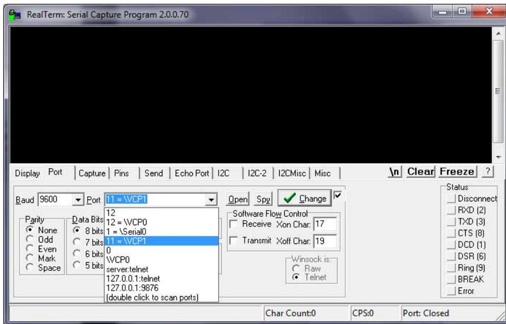
Figure 15: Realterm Port Settings for FTDI Device.
