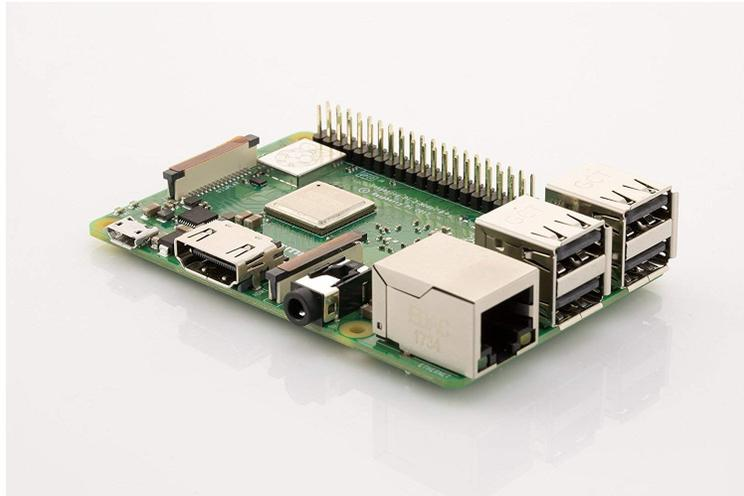
Figure 3: Raspberry Pi 3B+ Model.
