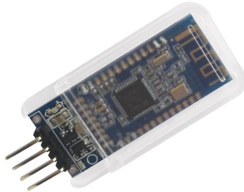
Figure 8: HM-10 Module from DSD Tech
