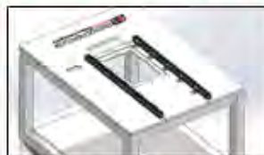
Sliding table design with rail and L-bracket supports
