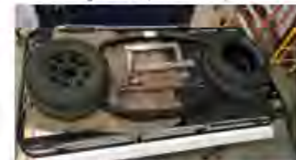
Figure 6 - Static Load Testing (600lb load)
