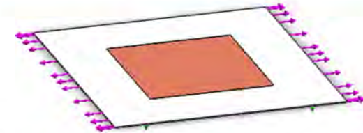
Figure 1: Forces Applied to Create a Maximum Displacement of 10mm ΔL
