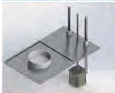
Figure 4: The Platform is an aluminum plate with a small cut-out for a glass surface or petri dish. This allows the user to print directly on to the proper surface for use. The platform is actuated vertically allowing the user to print an object up to 6 in tall. This 8 in. by 8 in. by 6in print volumes is one of the largest on the bioprinting market today.
