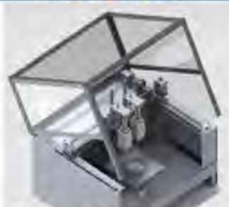
Figure 1: The Cover is made of an aluminum frame and acrylic panels, while the main frame of the printer is made of aluminum panels. The acrylic allows the user to look into the printer during printing to ensure a quality print is being made. Panels keep contaminants out of the printer while a Hepa filter allows only clean air into the printer.
