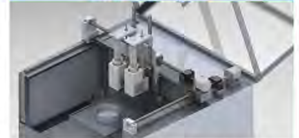
Figure 3: The Planar Motion System is composed of two lead screws with anti-backlash nuts to reduce vibrations. The extruder is moved from left to right by one motor and lead screw while that mechanism is moved front to back by a second motor. The planar motion system allows tissue to be printed over an 8 in. by 8 in. region.
