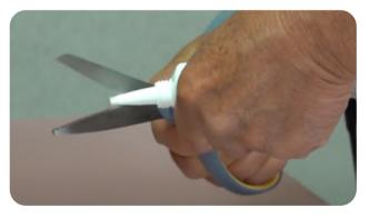
2. Cut the caulk tube at a diagonal to help spread out the caulk [Video 1, 21:25]
