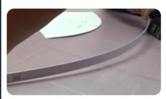
1. Use a flexible ruler to connect two endpoints of the curve [ <u>Video 1</u>, 7:08 ]
