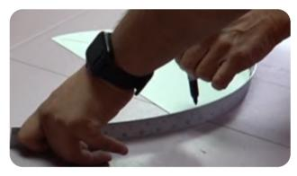
3. Mark the curve created by the ruler around the radius template Note: If bigger than the radius, you are good. If less than the radius, make the ruler wider and mark it
