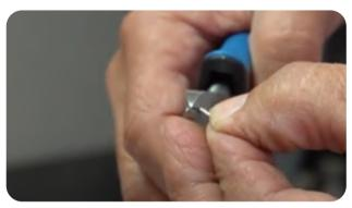
5. Clip both ends of the jointers using the back side of the track cutter to make it easier to go in and not have to cut an extra webbing from the track.
