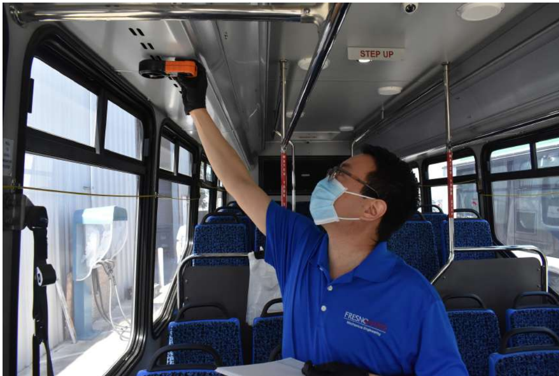
Figure 2. Airspeed from HVAC Ducting being Measured
