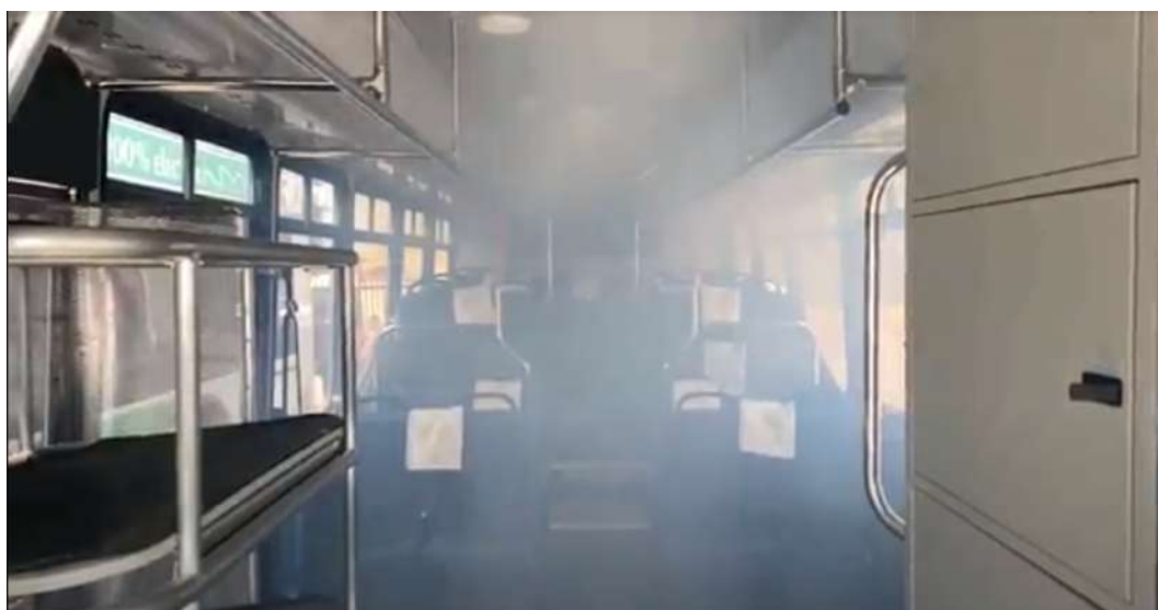
Figure 10. Experimental Steam Visualization of the Interior Stationary Bus A Viewing from the Front
