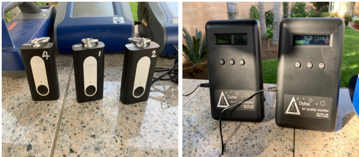
Figure 20. Low-cost Particulate Matter Air Sensors. (Left) AtmoTube Pro. (Right) Dyllos DC1700
