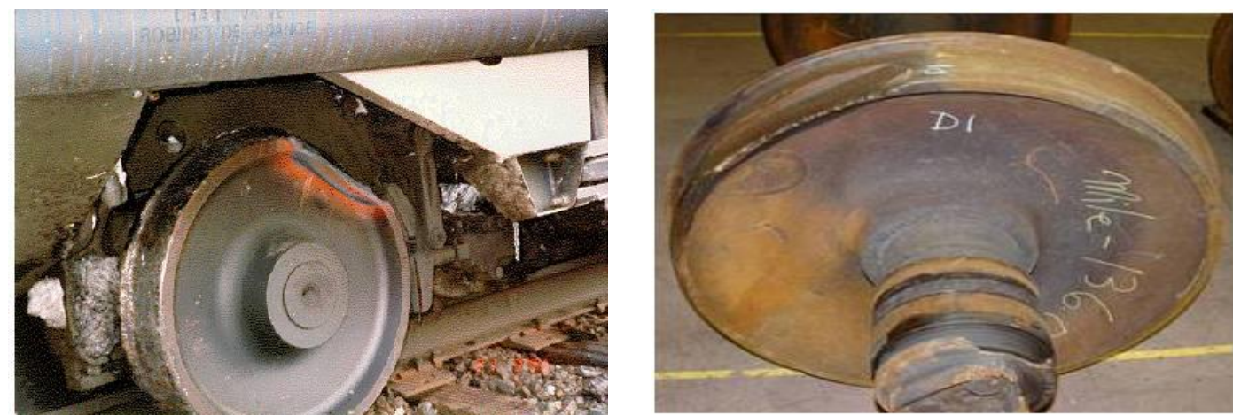
Figure 2. Wheel flat irregularities causing extreme loading conditions, (Transportation Safety Bureau of Canada, 2007)
